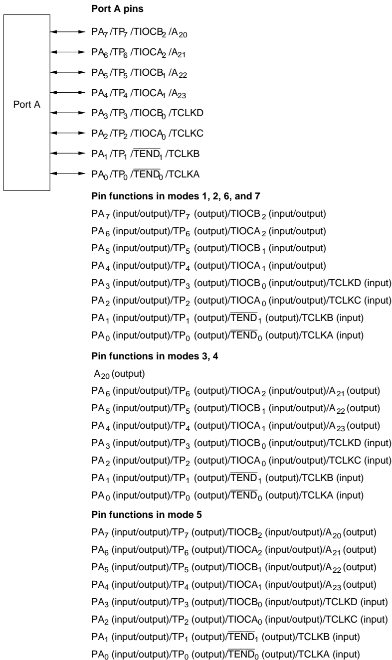
Figure 8.10 Port A Pin Configuration
